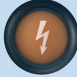
**3** When instructed by the device, press the orange Shock button.
